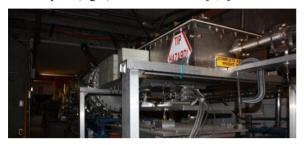
Figure 7: Collimator wakefield chamber test allows an exchange of collimators and adjustment of jaw aperture [8,9].
