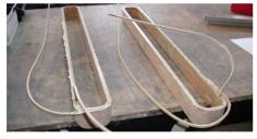
Figure 3: Kicker magnet copper coils.
