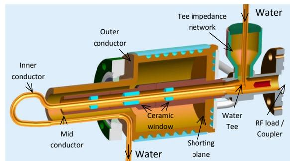
Figure 1: Cross section of damper geometry with capacitive ceramic elements.
