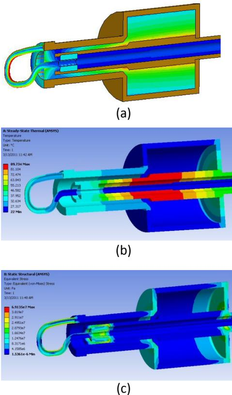
Figure 4: Rf and mechanical simulation results for the low-frequency stepped-impedance damper: (a) magnetic field magnitude, (b) thermal distribution, and (c) Von Mises stress.
