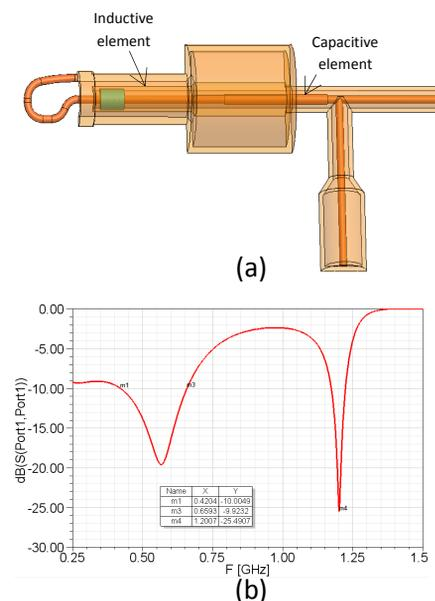
Figure 3: Low-frequency damper with a 3-element, stepped-impedance Tchebychev filter: (a) low-frequency damper with water tee, and (b) broadband frequency response.
