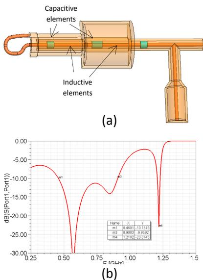
Figure 2: Low-frequency damper with a 5-element, capacitively loaded Tchebychev filter: (a) low-frequency damper with capacitive ceramic elements, and (b) broadband frequency response.
