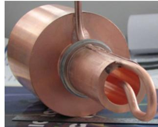
Figure 5: Prototype damper coupling loop and outer conductor after Glidcop brazing.
