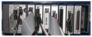
Figure 3: NI cRIO with I/O modules installed.
