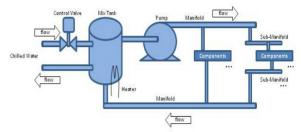
Figure 1: Drift tube linac water cooling system.
