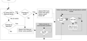
Figure 6: Valve logic diagram.
