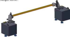
Figure 2: IFMS with the 4-m moving coil G10 board.
