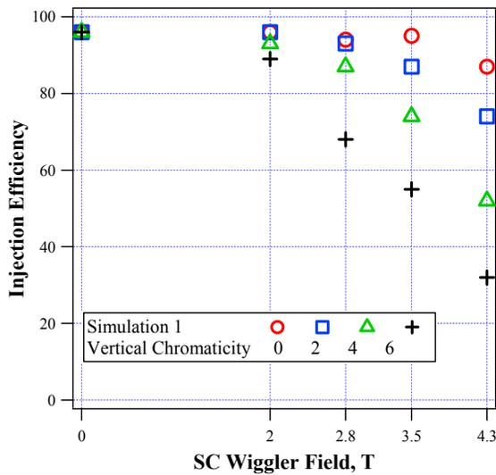
Figure 1: Simulation 1 and Injection efficiency for different BMIT wiggler fields and chromaticity.
