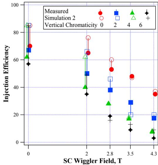
Figure 2: Simulation 2, Measurements, and Injection efficiency for different fields and chromaticity. (points are offset horizontally for clarity).
