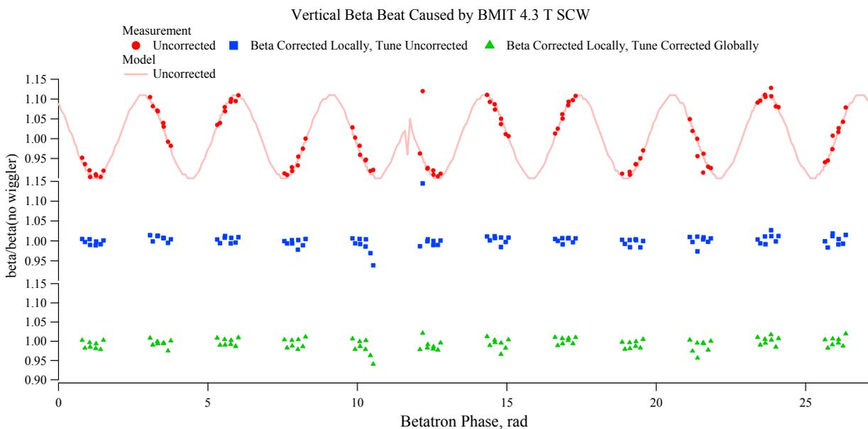
Figure 3: Measurements of the Vertical Beta Beat caused by a SCW at 4.3 T. Shown are the cases for uncorrected, local beta correction only, and local beta correction plus global tune correction.
