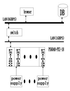
Figure 2: Whole structure of hardware.
