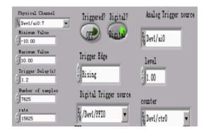
Figure 3: Settings interface of ADC card.
