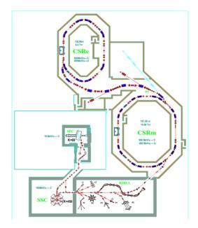
Figure 1: Overall layout of HIRFL-CSR.
