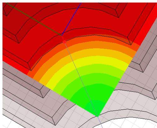
Figure 3: Plot of the magnitude of the magnetic field on a cross section of the beam tunnel showing the uniformity of the field around the azimuth. The variation of the colors shown is about 5 Gauss.
