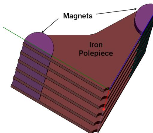
Figure 2: One quarter of a section of the PPM structure.
