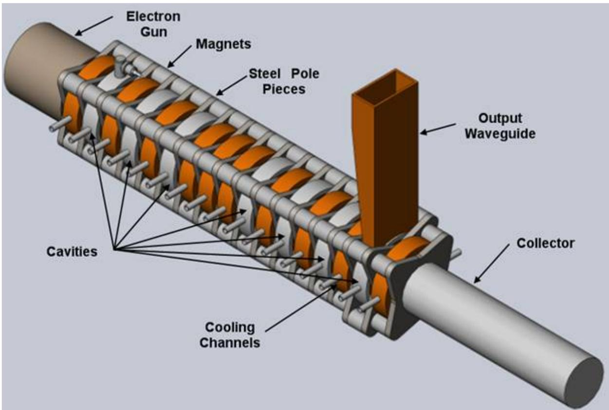
Figure 1: Solid model of the 100 kW S-Band klystron.
