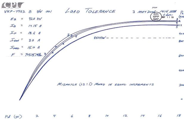
Figure 8: Load tolerance was measured at the factory with calibrated mis-matches. It shows the effect on the output due to load VSWR.
