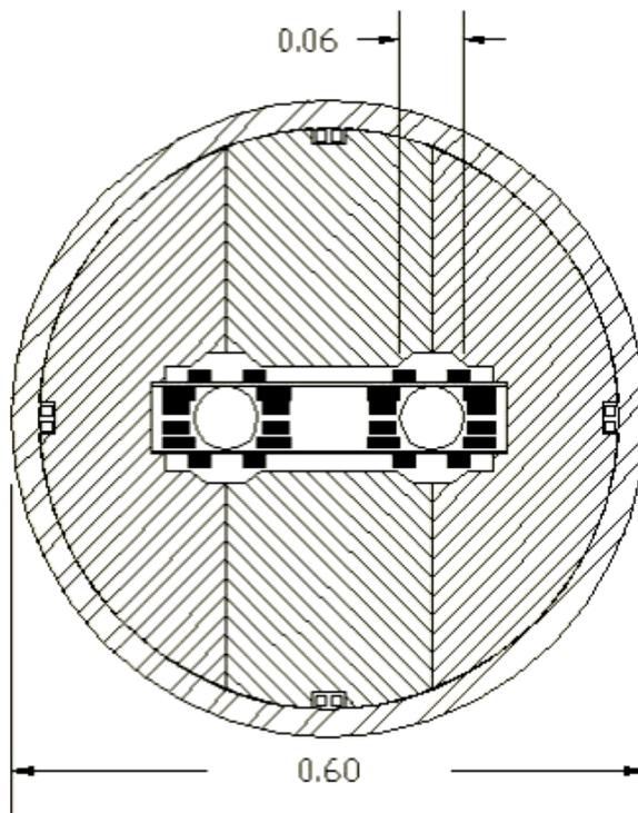
Figure 1: Cross-section of the block-coil Nb<sub>3</sub>Sn DS dipole.
