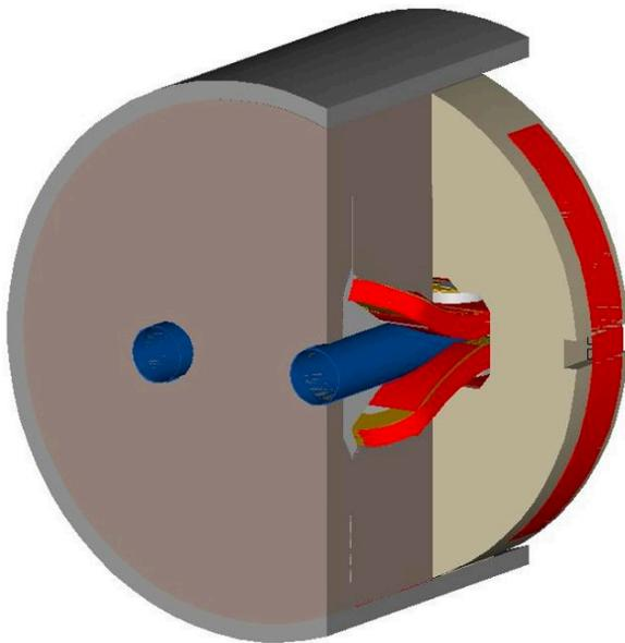
Figure 3: Isometric view of DS magnet end with cutaway, showing flared windings supported on 3-piece shoe assembly, bladder arrangement for isostatic preload of body and ends of all windings.
