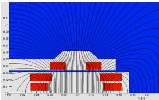
Figure 4: Calculated field distribution in DS dipole at 11.4 T.
