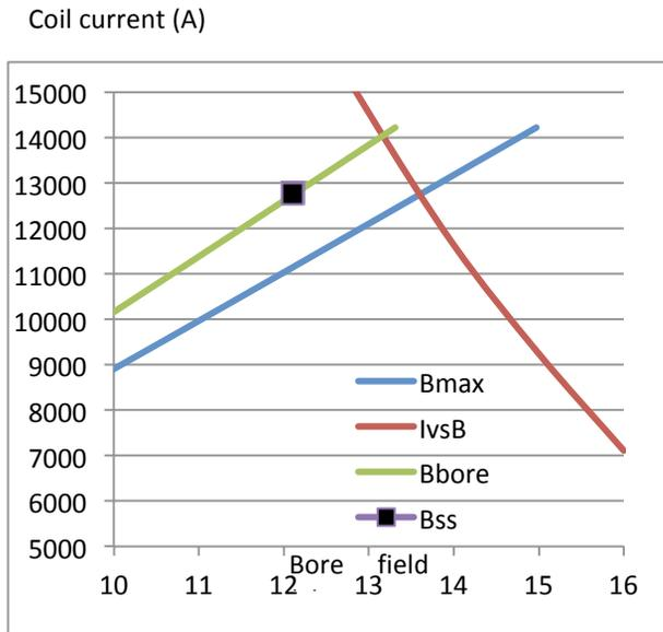
Figure 2: Load line for DS dipole.
