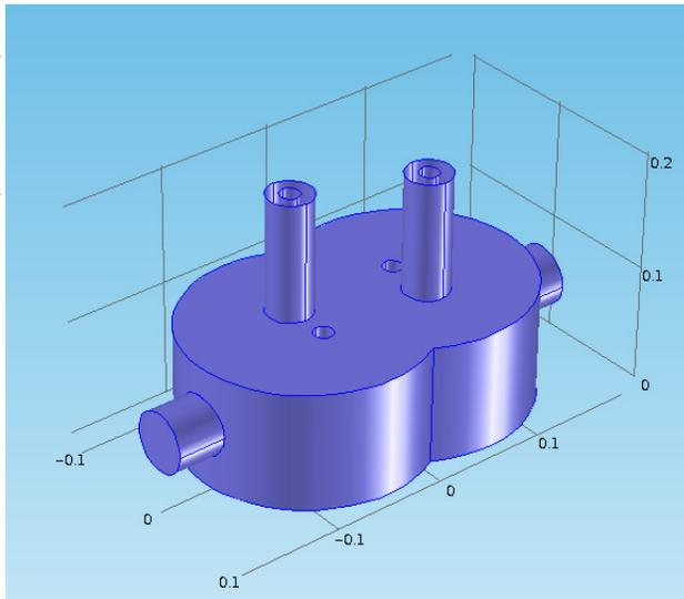
Figure 7: A two cell hybrid crab cavity with offset input power couplers
