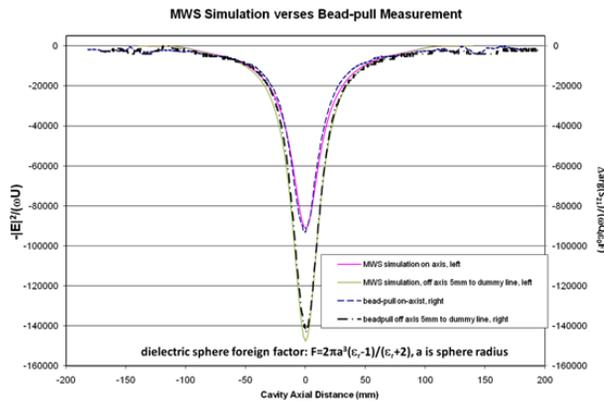
Figure 6: Test results of the bead pull measurement compared to MWS calculations
