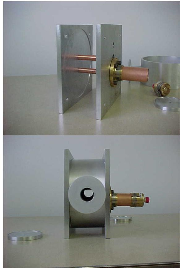
Figure 1: Pictures of the hybrid crab cavity prototype cold test components.
