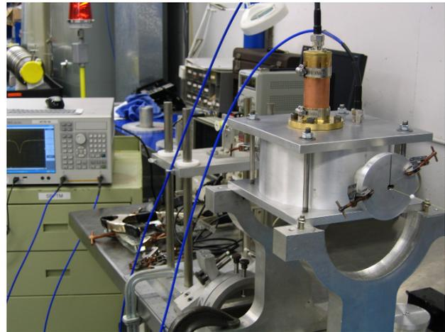
Figure 4: The cold test cavity is shown in the JLAB test lab for the bead pull measurement
