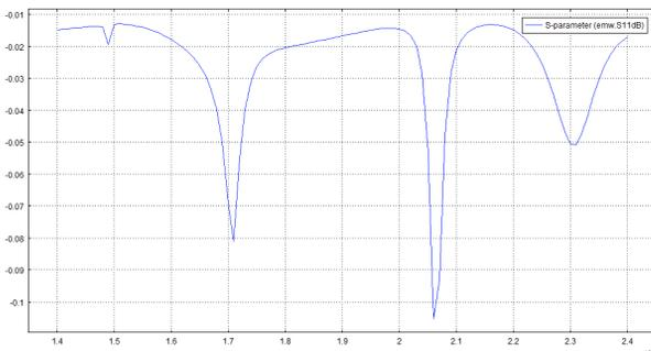
Figure 3: Calculations of S11 from 1.4 to 2.4 GHz.
