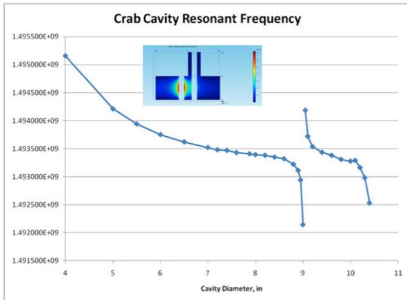
Figure 2: The resonant frequency of the half-wavelength bar as a function of cavity diameter.
