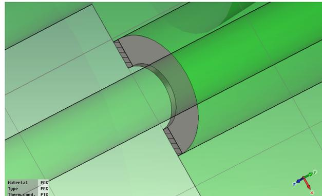
Figure 5: The coax iris used in the measurements
