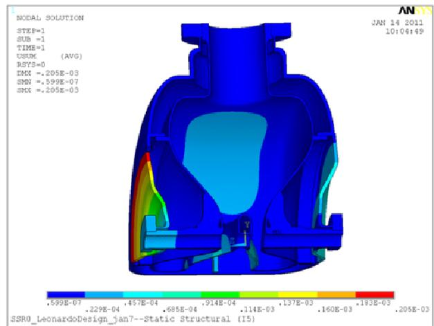
Figure 4: Optimization of the position of the circular rib to minimize df/dP. The left beam pipe is connected with bellows to the helium vessel, the right one is welded. This analysis produced a result of 5 Hz/torr.
