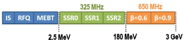
Figure 1: The Project X CW linac.
