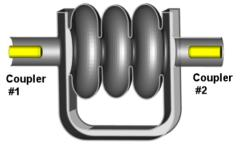
Figure 7: The STWR feeding scheme trough beam pipe.
