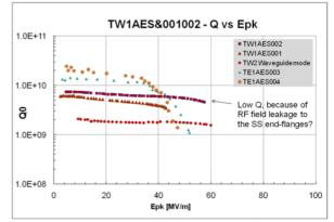
Figure 3: Quality factor vs. surface electric field for 1-cell TW cavities (TW1AES001, TW1AES002) in comparison to TESLA-like TE1AES 1-cell cavities.
