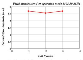
Figure 5: The field distribution for operation mode in the 3-cell TW cavity
