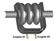
Figure 6: The STWR feeding scheme trough waveguide couplers.
