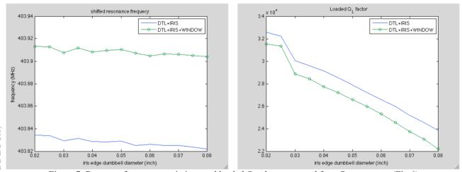
Figure 7: Resonant frequency variations and loaded Q values extracted from S-parameters (Fig.6).
