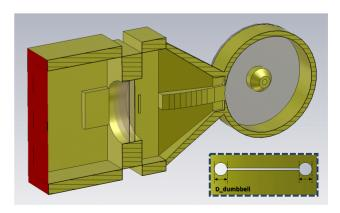
Figure 1: 3-D EM model on assembly of DTL tank cell, waveguide iris taper transition and WG window.
