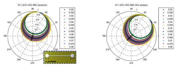
Figure 6: S11 of DTL/IRIS (left) DTL/IRIS/Window model (right) with various slot dimensions (D\_dumbbell).
