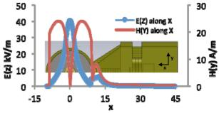
Figure 3: E(z) and H(y) field plots along the RF propagation axis (x-direction, y=z=0). Beam axis (zdirection at x=y=0), drift tube center has maximum E and minimum H field. E field drops rapidly at the coupling slot interface.
