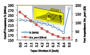
Figure 2: Double-ridge waveguide iris transition model and its cross-sectional port properties (cutoff frequency f<sub>c</sub>, port impedance Z<sub>re port</sub>). Each point is based on CST model of waveguide with cross-section along x direction.
