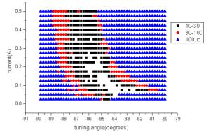
Figure 2: Results of 500 000-turn simulations of 450 macroparticles.  $\blacksquare$ : mild instability, where the energy spread exceeds its natural value by (10-30)%;  $\bullet$ : moderate instability, where the energyspread has increased by (30-100)%;  $\blacktriangle$ : strong instability, where the energy spread has increased more than 100%.
