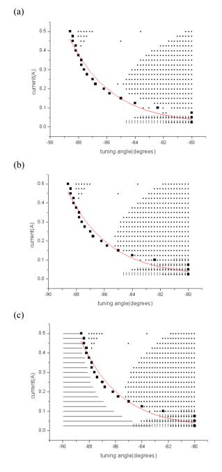
Figure 1: (a) Robinson in stabilities are predicted without consideration of mode coupling. A solid curve shows the parameters for optimal bunch lengthening, in which case the linear synchrotron frequency is zero. Vertical line: dipole instability; Spot: quadrupole instability. (b)Dipole-quadrupole mode coupling is included. Vertical line: coupled-dipole instability; Spot: coupled-quadrupole instability. (c)Coupled bunch instability is included. Horizontal line: coupled bunch instability.
