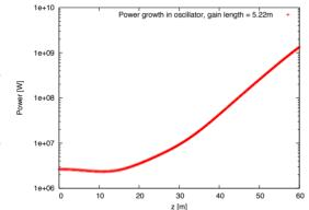
Figure 4: Power evolution inside the high gain FEL at the OFFELLO saturation.
