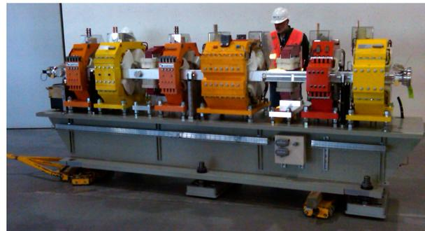
Figure 9: First completed magnet-vacuum girder of the NSLS-II Storage ring carrying magnets, vacuum chamber, and beam instrumentation hardware, cooling manifolds, support systems and cable trays.
