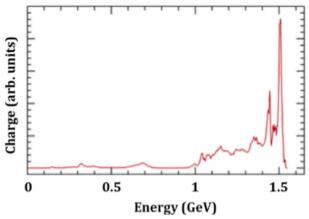
The electron energy spectrum from a 2D Figure 8: OSIRIS simulation for a 100 TW LWFA with staged injection in 1.5x10<sup>18</sup> cm<sup>-3</sup> density plasma
