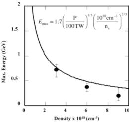
Figure 2: Measured electron energy verses plasma density. The theory curve is for 65 TW of laser power. Data taken from Ref. [7, 8]
