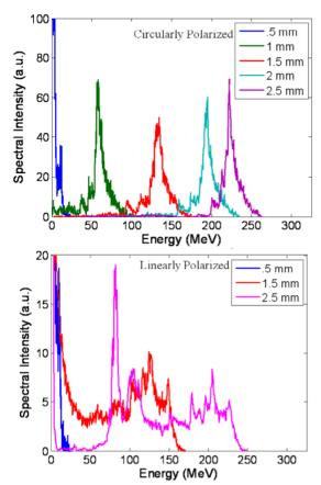
Figure 6: 2D OSIRIS simulation results comparing the accelerated electron spectra with circular polarization and with linear polarization. With circular polarization injection is turned off early in the simulation when the electric field falls below the ionization threshold. In the linear case ionization injection continues throughout the simulation resulting in a large energy spread.
