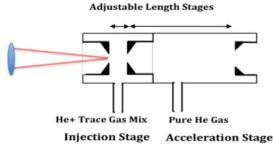
Figure 7: Illustration of staged injection concept.
