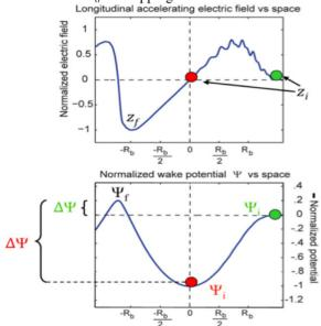
Figure 3: On axis line outs of longitudinal electric field and the wake potential verses z location in units of  $R_b$  for 2D OSIRIS simulation with  $n_e = 1.4 \times 10^{19}$  cm<sup>-3</sup>,  $a_0 = 2.5$ . The figure illustrates how ionization trapping increases the potential seen by the electrons (shown in red and green) when born closer z = 0. Ref. [10].
