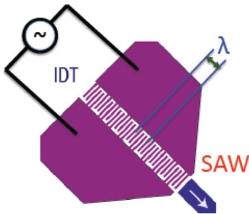
Figure 1: Schematic layout of SAW generation.
