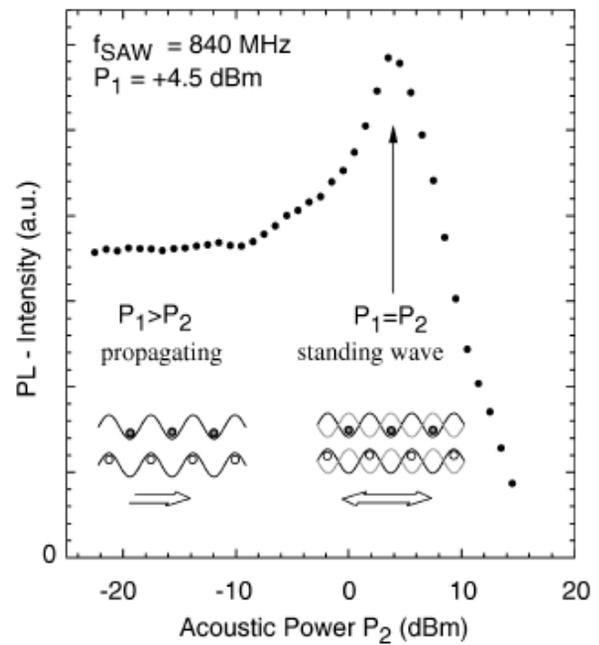
Figure 3: Photoluminescence is enhanced for standing SAW compared to propagating SAW.
