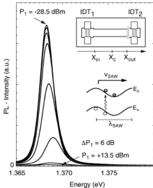
Figure 2: Photoluminescence spectra of a single 10 nm wide InGaAs/GaAs quantum well structure for different acoustic powers. The optical excitation occurs at the site  $x = x_c$  with an intensity of  $10 \text{ mW/cm}^2$  and laser wavelength =  $780 \text{ nm}$ . The inset schematically depicts the sample design with two interdigital transducers (IDT) and the storage of optically generated excitons in the potential of a surface acoustic wave.
