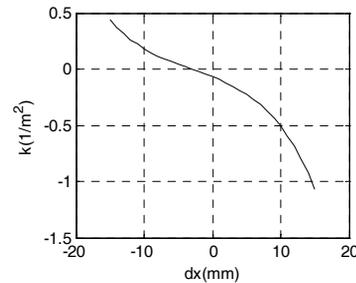
Figure 3: Quadrupole term v.s. orbit distortion in B2.
