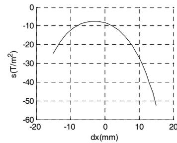
Figure 2: Sextupole term v. s. orbit distortion in B2.
