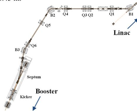
Figure 1: LTB layout from LINAC to Booster
