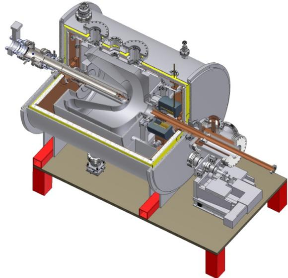
Figure 2: SRF Gun and Cryostat.
