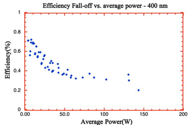
Figure 2: Lasing efficiency as a function of output power
