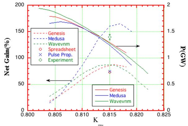
Figure 1: Modeled gain &amp; power (lines), 1D calculated gain (points), and measured gain (point).
