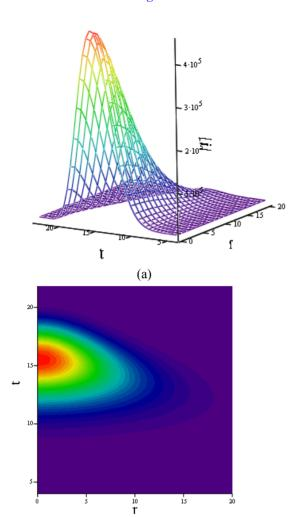
Figure 2 The amplitude of amplified current density modulation as calculated from eq. (29). The snapshot is taken at  $\hat{z} = 21$  with  $\hat{\sigma}_t = 1.37 \times 10^{-5}$ ,  $\hat{\Lambda}_p = 0$ ,  $\hat{\sigma}_\perp = 2.32$  and  $\hat{q} = 0.1$ . (a) the amplitude of current modulation as a function of transverse spatial radius and longitudinal arrival time; (b) contour plot of (a).
