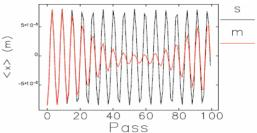
Figure 1: The beam center change with single and multi particles tracking.
