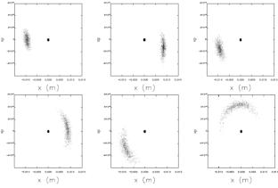
Figure 2: The injected beam and stored beam beam horizontal phase space in the first 15 turns (number increase from left to right for every 3 turns).
