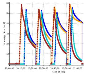
Figure 6: RF voltage scan at  $\gamma$ =4.1. Four stores with 450, 300, 200 and 100kV RF voltage per ring, subsequently. Upper (blue and yellow) curves – total current in the Blue and Yellow rings; lower (light blue and brown) curves - bunched beam current.
