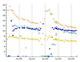
Figure 5: Vertical axis: horizontal and vertical emittance (95% normalized [mm mrad]) in Blue and Yellow ring for two short stores at  $\gamma$ =6.1 with collisions starting at 11:03 and 11:18, respectively.
