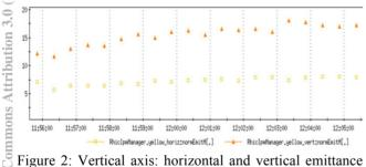
Figure 2: Vertical axis: horizontal and vertical emittance (95% normalized [mm mrad]) for beam in Yellow ring without collisions at  $\gamma$ =6.1; horizontal axis: clock time.
