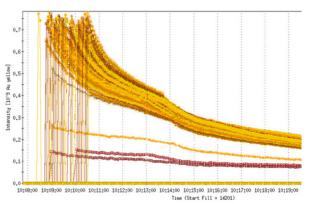
Figure 4: Intensity (x10<sup>9</sup>) of individual bunches in Yellow ring before and after collisions at  $\gamma$ =4.1 (bunches were injected in the Blue ring and put into collisions at about 10:14 clock time on horizontal axis).
