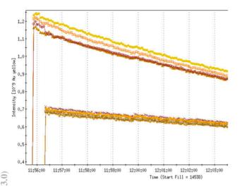
Figure 1: Intensity  $(x10^9)$  evolution of several bunches at  $\gamma$ =6.1 without collisions.
