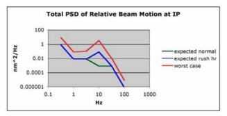
Figure 9: Power spectrum of beam relative motion at IP. Includes ground motion, magnet supports, IR cantilevers, and beam feedback.
