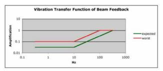
Figure 8: Performance of fast luminosity feedback system
