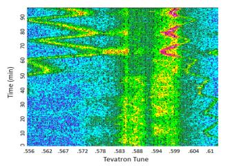
Figure 5: Horizontal 21 MHz Schottky spectrum of proton beam measured at 980 GeV (see text).
