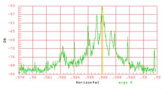
Figure 4: Horizontal 21 MHz Schottky spectrum of proton beam measured at 980 GeV measured 09/29/2002.
