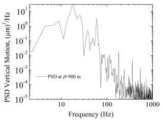
Figure 3: Low frequency power spectral density of the vertical orbit oscillations.
