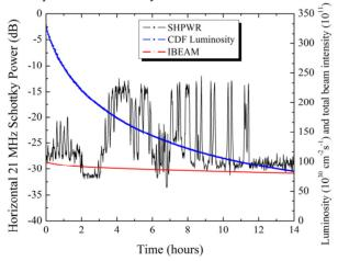
Figure 6: Variation of the horizontal 21 MHz Schottky power during 14-hours colliding run #8548 (March 9, 2011).
