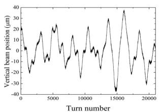
Figure 1: Vertical position of the proton bunch #11 at the beginning of HEP store #6214 (October 2008), measured at the VB11 location with  $\beta_v$ =900 m.
