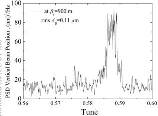
Figure 2: Power spectral density of the vertical betatron oscillations (FFT of the data presented in Fig.1).
