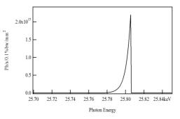
Fig. 4: Energy dependency of flux density for min x-ray spot case at CEBAF
