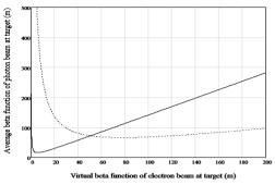
Fig. 1: Average beta function of photon beam at target (solid line), electron beam input beta function (dashed line) versus virtual beta function of electron beam at target
