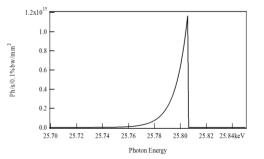
Fig. 3: Energy dependency of flux density for min input case at CEBAF
