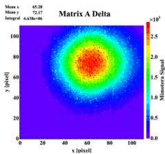
Figure 1: Profile of one shot of antiprotons in the Mimotera detector. Mean values in x- and y-direction are displayed, as well as the integral of the signal over the whole detector surface [3].
