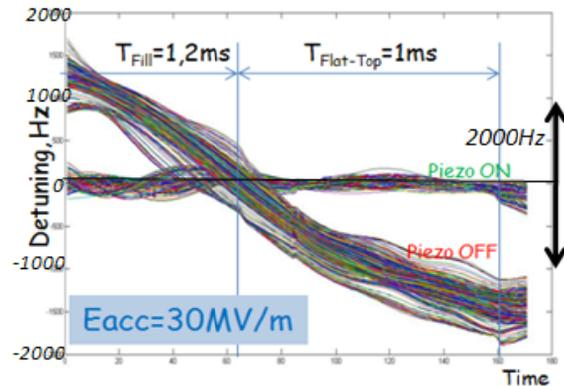
Figure 3: Detuning of a 325 MHz Spoke Resonator with and Without Compensation
