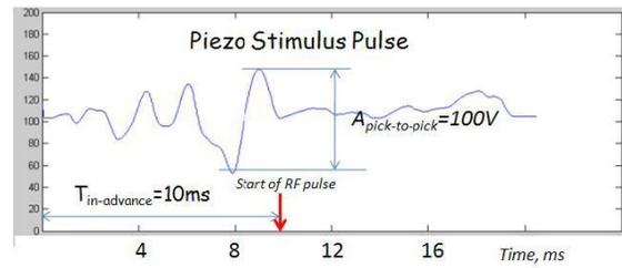
Figure 2: Compensation Piezo Wave Form for the Elliptical Cavity
