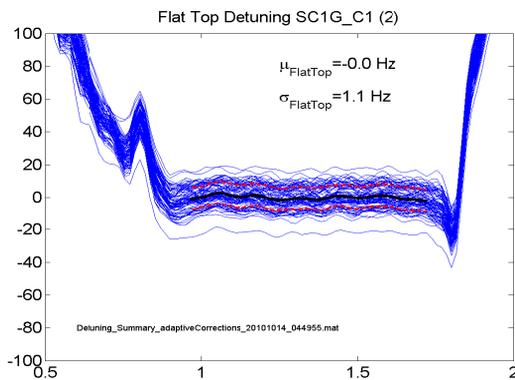
Figure 6: Detuning a Blade Tuner Equipped Cavity Installed in the S1-G Cryomodule at KEK
