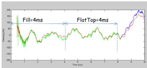
Figure 5: Detuning in a Nine-Cell Elliptical Cavity Driven by an 8 ms RF Pulse.
