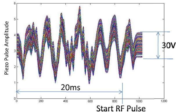
Figure 4: Compensation waveforms for the Spoke resonator.
