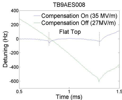
Figure 1: Lorentz force compensation in a nine-cell elliptical cavity at 35 MV/m.
