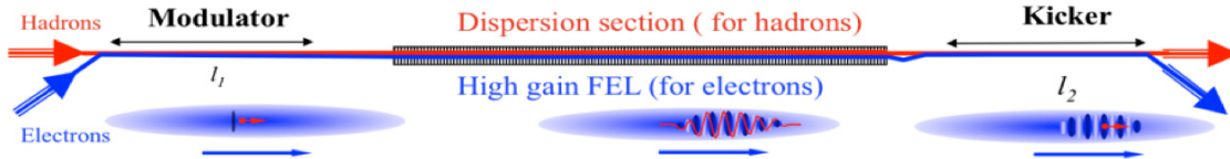
Figure 3: Economic version of coherent electron cooler, wherein electrons and hadrons are not separated transversely.
