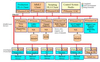
Figure 1: System Architecture.
