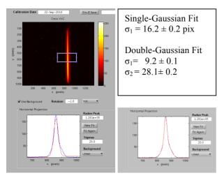
Figure 5: The total radially polarized OTR image (TOP) for a vertical band focus with the single-Gaussian (L) and double-Gaussian fits (R) to the projected profiles.
