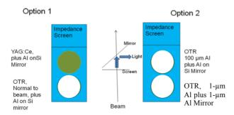
Figure 3: Schematic of the converter screen options considered for the prototype tests. Option 1 was the initial case tested and reported here.
