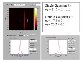
Figure 6: The vertically polarized OTR image (TOP) for a vertical band focus with the single-Gausssian (L) and two- Gaussian fits (R) to the projected profiles.
