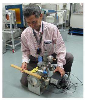
Figure 2 showing the entrance window, vacuum port with calibrated leak valve and vacuum gauge.
