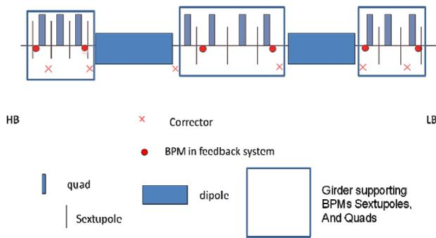
Figure 2: BPMs, Quads and correctors for FOFB [8].
