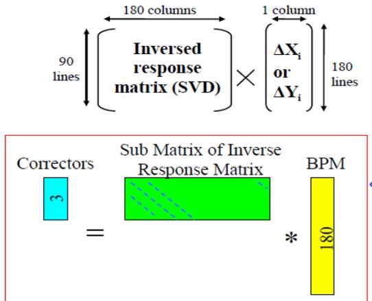
Figure 4: Orbit feedback computation [9].
