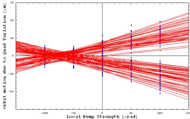
Figure 3: "Bowtie plot" method for BBA [8].
