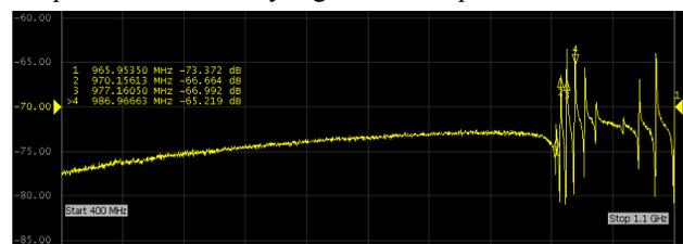
Figure 6: Measured S21-parameter in the S2 production chamber with RF shielding inside (logarithmic scale). Input and output signals are taken from upstream BPM.
