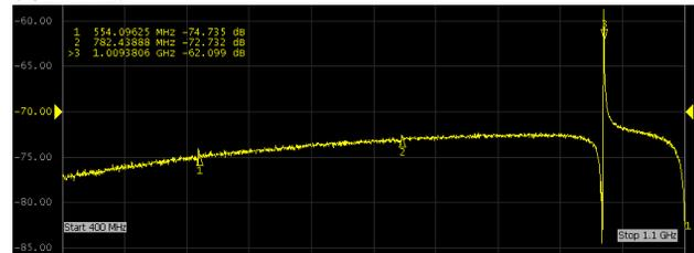
Figure 5: Measured S21-parameter in the S4 production chamber with RF shielding inside (logarithmic scale). Input and output signals are taken from downstream BPM.
