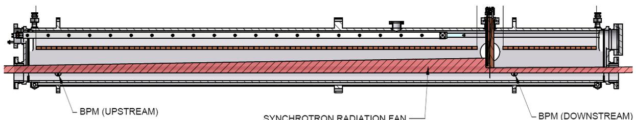
Figure 4: S4 chamber with RF shielding inside. The red shaded region represents the synchrotron radiation fan.
