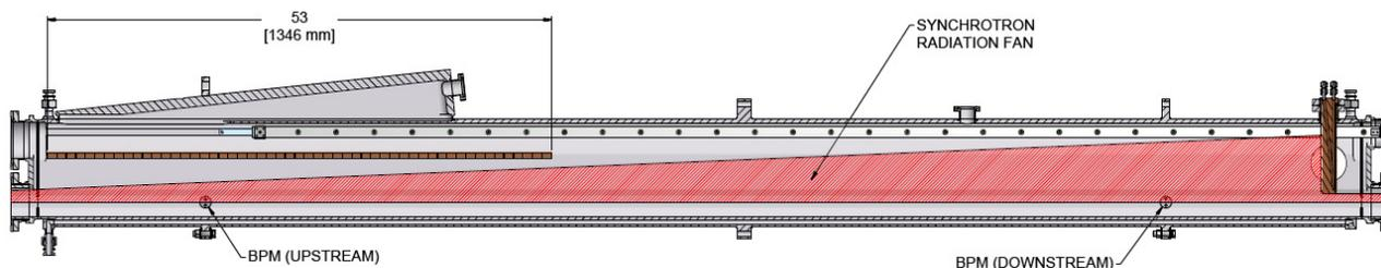
Figure 7: S6 even multipole vacuum chamber with RF shielding inside. The red shaded region represents the synchrotron radiation fan. Flexible BeCu RF shielding is  $1346\text{mm}$  long.
