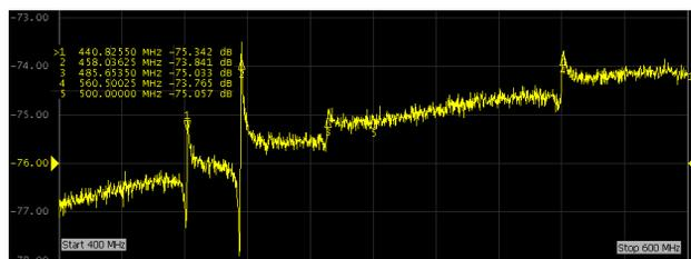
Figure 9: Measured S21-parameter in the S6 odd production chamber ( $3445\text{mm}$  inner length) with RF shielding inside (logarithmic scale). Input and output signals are taken from downstream BPM.
