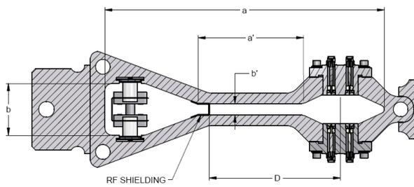
Figure 2: NLS-II multipole vacuum chamber profile.
