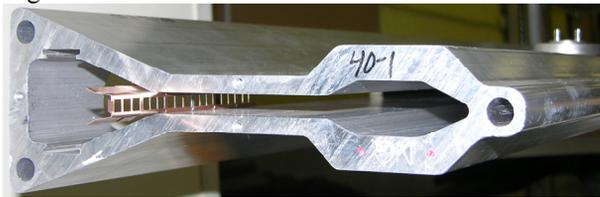
Figure 3: Flexible BeCu RF shielding with 50% of opening inside the multipole vacuum chamber. The thickness of the RF shielding is 0.25mm.
