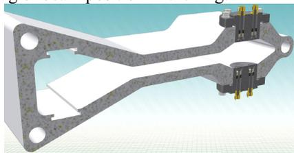
Figure 1: NSLS-II multipole vacuum chamber profile.
