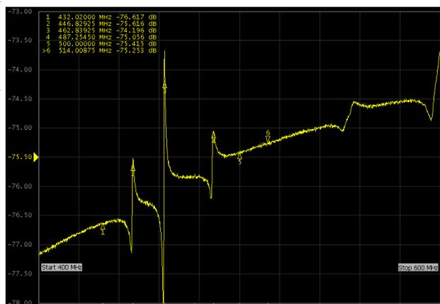
Figure 8: Measured S21-parameter in the S6 even production chamber ( $3559\text{mm}$  inner length) with RF shielding inside (logarithmic scale). Input and output signals are taken from downstream BPM.
