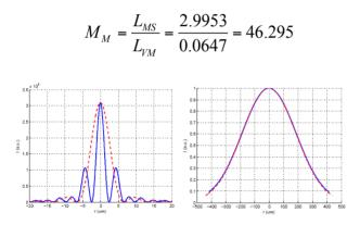
Figure 6: (a, left) Diffractogram with point virtual source (b, right) Image on the screen obtained from numerical study.  $L_{VM} = 64.720$  mm,  $L_{MS} = 2.995280$  m.
