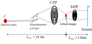
Figure 1: Schematic view of X-ray imaging at 1B2 beam line in Pohang Light Source (PLS). The energy of X-ray after monochromator is 6.95 keV. The distance from the electron beam to the virtual image  $L_{EV}$  is 24.4 m. The distance from the virtual image to the detector  $L_{VS}$  is 3.06 m. The vertical electron beam  $\sigma$  is about 35 µm.
