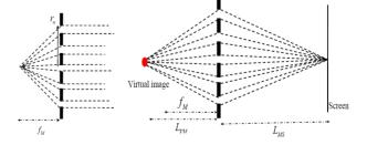
Figure 5: (a, *left*) Design of MZP. The focal length is 63.55 mm. The zone number is 571. The radius of the outmost ring  $(r_N)$  is 80  $\mu$ m. (b, *right*) Schematic view for the imaging of electron beam on the screen by MZP.
