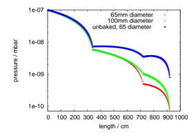
Figure 4: Pressure along the new beamline.
