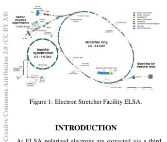
Figure 1: Electron Stretcher Facility ELSA.
