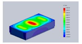
Figure 2: FEM analysis showing the deformation of the mirror surface.
