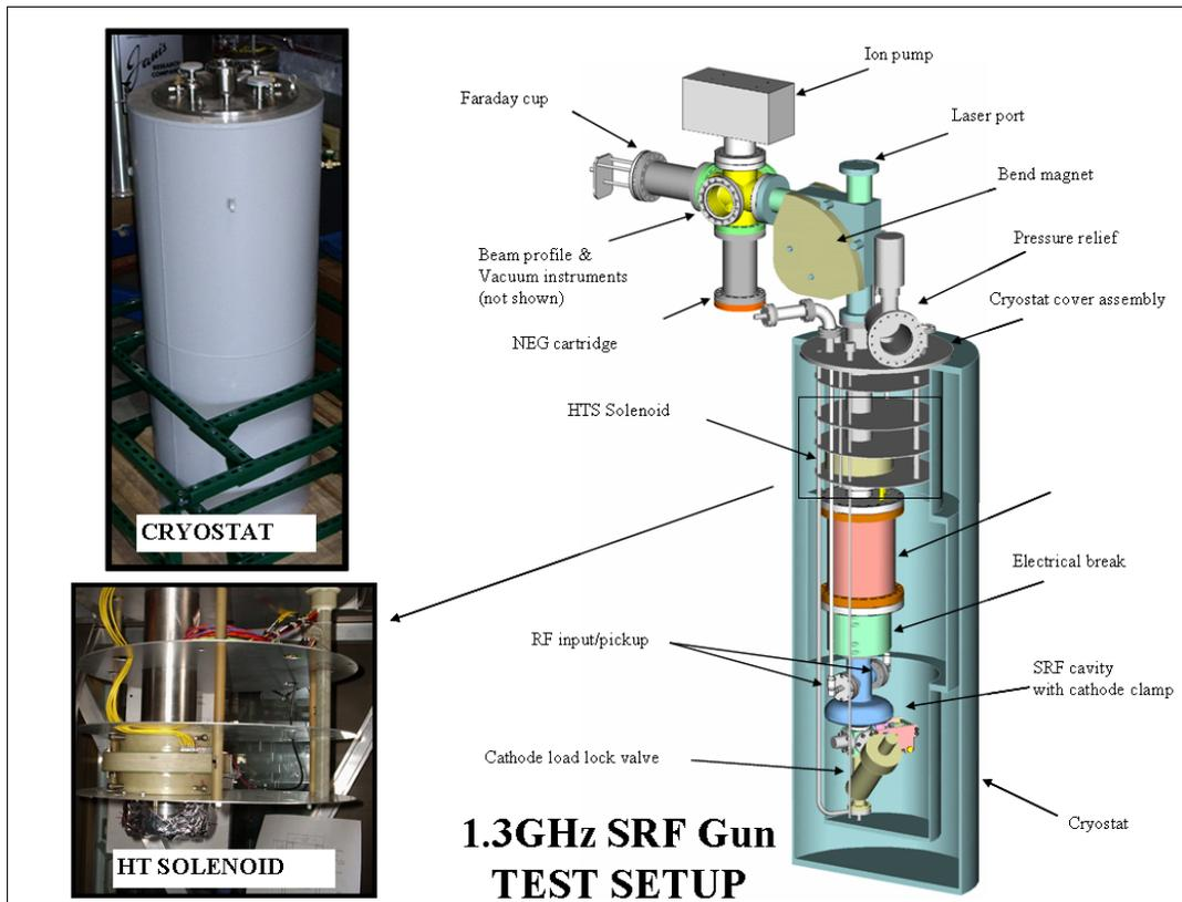
**1.3GHz SRF Gun TEST SETUP**
