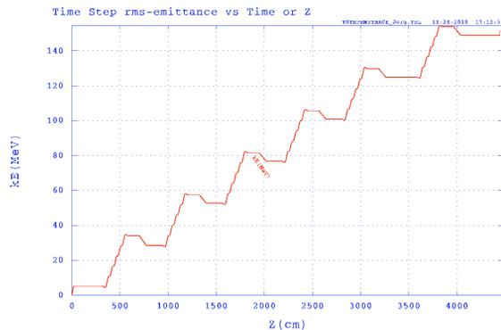
Figure 6: Beam energy evolution through six sets of subsequent fundamental and 3rd harmonic cavities.
