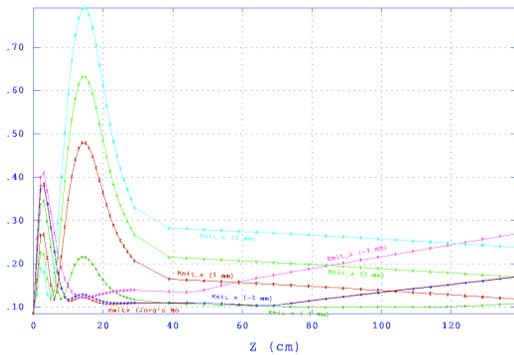
Figure 5: Gun axial emittance profiles varying the cathode location by  $\pm 3 \text{ mm}$ .
