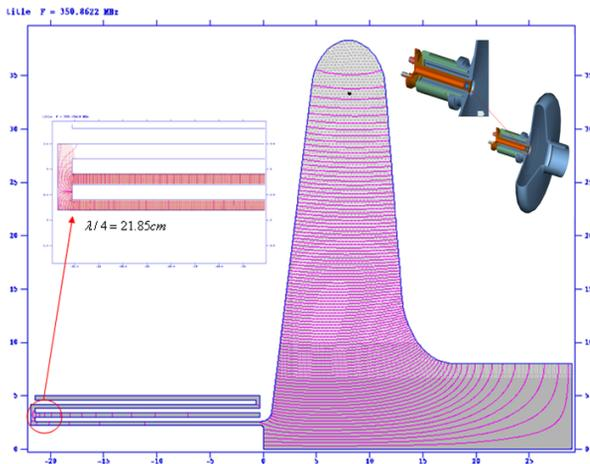
Figure 4: 350 MHz SUPERFISH half-cell SRF cavity with the optimized 21.85 cm QWC geometry (upper left) and HTS (upper right).
