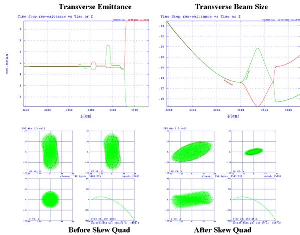
Figure 7: PARMELA beam evolution (upper) and phase space plots (lower) for the pre skew quad round (left) and post quad rectangular beams (right).
