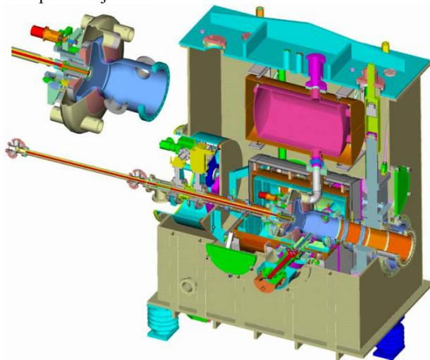
Figure 3: 703.75 MHz photocathode SRF gun cryostat and its half-cell cavity in the upper left detail.
