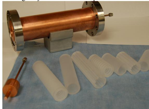
Figure 5: Example of manufactured quartz tubes: longitudinal and transverse grooves, various lengths, smooth tubes. Waveguide and mode launchers for bench test.
