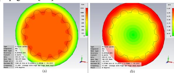
Figure 2: The magnitudes of the electric (a) and magnetic (b) fields of the  $TM_{01}$  mode in an 11.424 GHz longitudinally grooved quartz based DLA structure.
