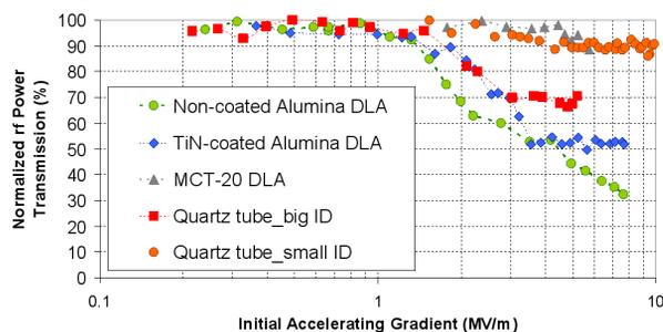
Figure 1: Summary of high power test results of dielectric loaded accelerating structures (AWA-NRL) [1].
