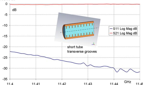
Figure 7: Bench test measurement (S-parameters) of a transverse-grooved structure.
