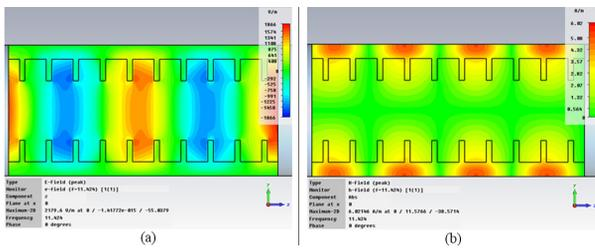
Figure 3: The magnitudes of the electric (a) and magnetic (b) fields of the  $TM_{01}$  mode in an 11.424 GHz transversely grooved quartz based DLA structure.
