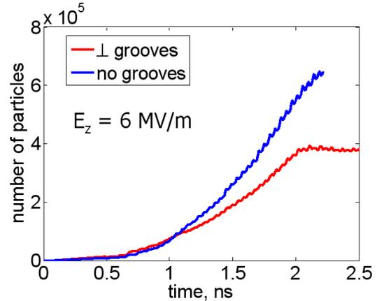
Figure 4: Comparison of the multipactor development for a smooth tube vs. a tube with transverse grooves.
