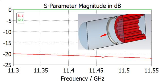
Figure 6: RF matching from an empty waveguide into waveguide loaded with a dielectric cylinder with longitudinal grooves. The metal bump position and size is optimized to provide perfect matching at 11.424 GHz for a particular tube geometry.
