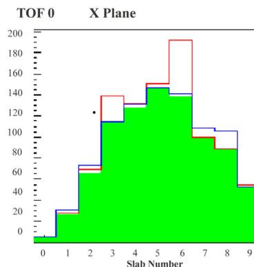
Figure 4: Histogram showing the slab hits due to PMT coincidence (green), as well as the TDC signals for PMT0 (red) and PMT1 (blue) for all slabs in the  $x$  plane of TOF0.
