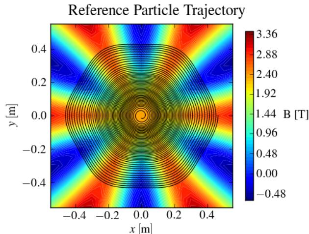
Figure 1: Trajectory of the reference particle with initial momentum of  $p = 180$  MeV/c and initial radius of  $r = 0.464$  m. The color contour behind the trajectory depicts the mid-plane strength of the magnetic field in Tesla.
