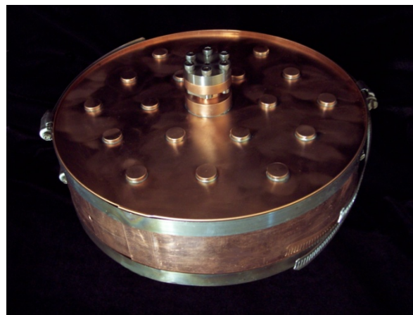
Figure 4: Copper prototype at 2.7 GHz.
