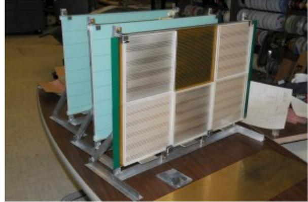
Figure 1: Prototypes of three TOF planes, each a 'Super-module' consisting of 6 tiles.
