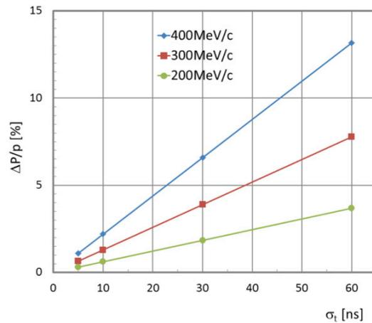
Figure 1: Momentum resolution of non-magnetic TOF spectrometer with various TOF resolutions ( $\sigma_t$ ) for incident beam momenta of 200, 300 and 400 MeV/c.
