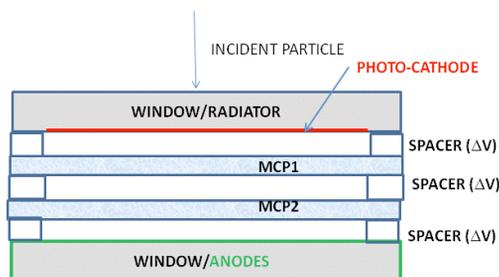
Figure 3: Cross section of a typical MCP-based planar TOF detector. Windows are shown in gray, MCPs are blue, photo-cathode and anode layers are red and green, respectively.
