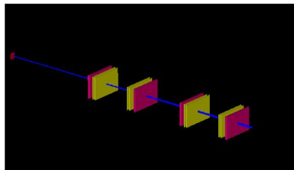
Figure 4: Two arm non-magnetic TOF spectrometer. The red planes are TOF detectors with time and space outputs.
