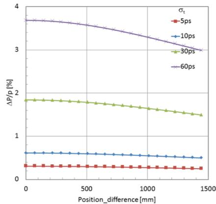
Figure 2: Position dependence of momentum resolution on TOF counters for 200-MeV/c beam. The position difference is defined as  $\sqrt{(x_2 - x_1)^2 + (y_2 - y_1)^2}$ , when a particle hits  $(x_1, y_1)$  and  $(x_2, y_2)$  on the detectors.
