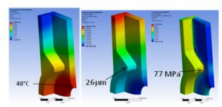
Figure 3: left) temperature distribution; right) stress analysis.
