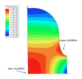
Figure 2: 2D profile of half cell of the DECA structure; electric field distribution is also shown.
