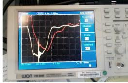
Figure 5: current (red) and voltage (yellow) pulses from Klystron in diode mode (no RF) for initial conditioning.
