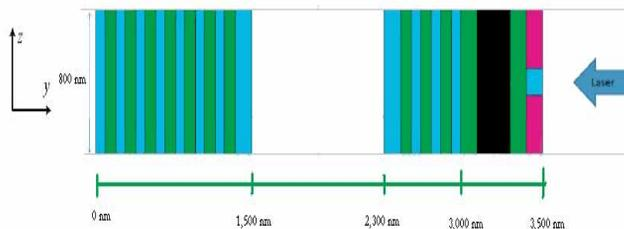
Fig. 1: One period of the MAP. The incident NIR laser propagates from right to left and electrons are accelerated along the  $z$ -axis. The structure is invariant in the  $x$  direction.
