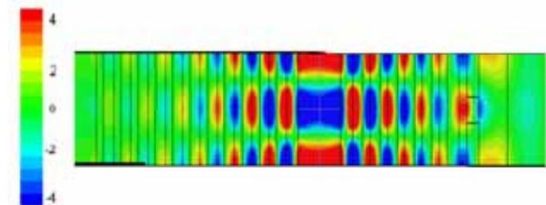
Fig. 3: Color field map of  $E_z$  in the  $\beta=0.875$  MAP exhibiting strong resonance, normalized to the drive laser amplitude. The laser propagates from right to left and electrons travel vertically through the cavity.
