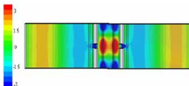
Fig. 5: Resonance in low beta simplified MAP due to two incident oppositely propagating lasers, normalized to the drive laser amplitude.
