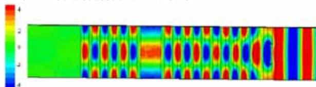
Fig. 2: Color field map of  $E_z$  in the relativistic MAP exhibiting strong resonance, normalized to the drive laser amplitude. Materials used are zirconia, silica, and hafnia. The laser propagates from right to left and electrons travel vertically through the cavity.
