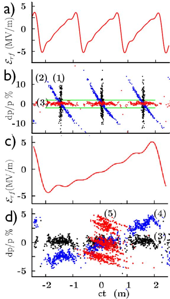
Figure 2: Longitudinal Merge: a) 201 MHz + harmonics; b) Initial Rotation (1)=initial, (2)=drifted, (3)=after rf<sub>1</sub>; c) 67 MHz + harmonics; d) Merge (3)=from above, (4)=rf<sub>2</sub>, (5)=drifted).
