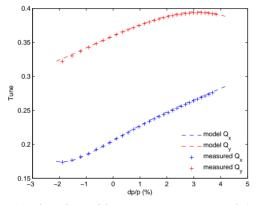
Figure 1: detuning with momentum: measured (crosses) model (continuous line barely visible below the crosses).
