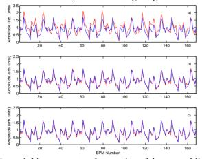
Figure 4: Measurement and correction of the spectral line  $Q_x - Q_y$  measured in the vertical plane: red – measured, blue - model, before correction (top) after one iteration (middle) after two iterations (bottom).
