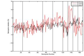
Figure 5: Sextupoles gradient variation required by the fit procedure outlined in the text; red for the case where one resonance was targeted; black for the case where two resonances were targeted.
