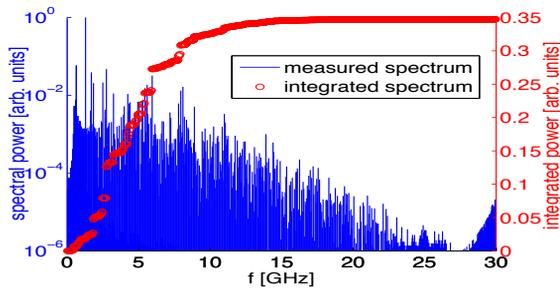
Figure 3: HOM spectrum excited by the beam as measured at one of the HOM loads. The integrated spectrum is plotted on the secondary axis.
