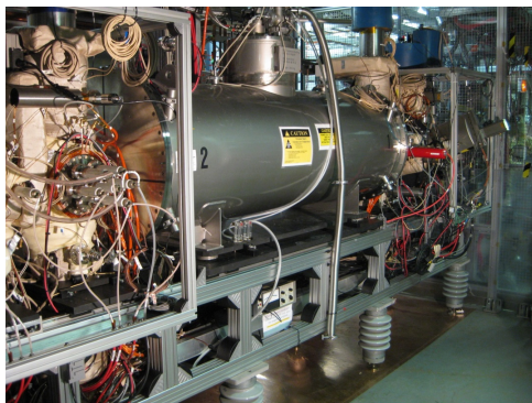
Figure 2: The EBIS source, with the 2m long superconducting solenoid producing a 1.5 m trap region.
